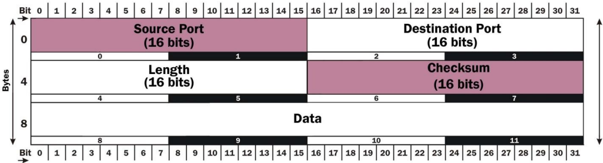
Figure 3.5-a: UDP Packet Header
